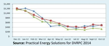
A quick visit to one of the stations on a cold February day revealed that the indoor temperature was 75°F and unit heaters were running despite a 60°F thermostat setting. By replacing broken thermostats in these three pump stations, the township is expected to save \$3,600 annually, with a payback in a matter of months. This initial (and easy) analysis of the pump station utility bills allowed PES to identify this simple and cost-saving energy-management opportunity.
