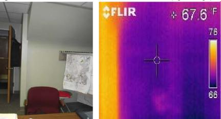
Figure 7: Air infiltration shown with infrared camera (right image)
