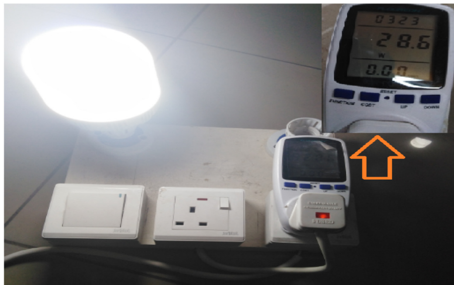
(b) Power consumption measurement of an LED bulb reading 28.6 W
